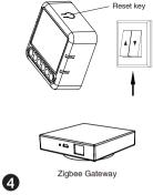
After the wiring of switch module is done, press the reset key for about 10 seconds or (1CH:turn on/off the traditional switch for 5 times,2CH:press the traditional switch for about 10 seconds) until the indicator light inside the module is flashing quickly for pairing.
